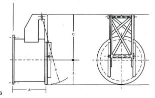
FLAT BAR GATE HANGER ASTM A-36
