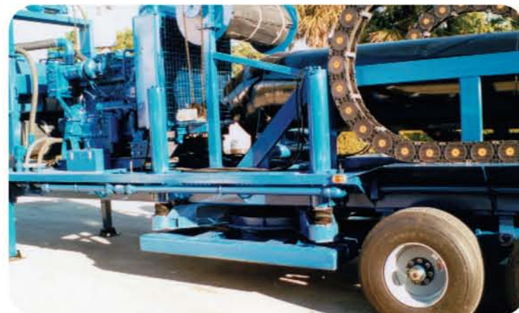
The turntable mechanism in traveling position.
